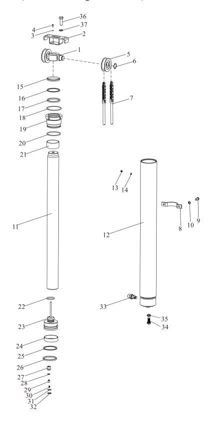
前起升油缸(三节全自由) Front Lift Cylinder (Full Free 3-Stage Mast KZM)
