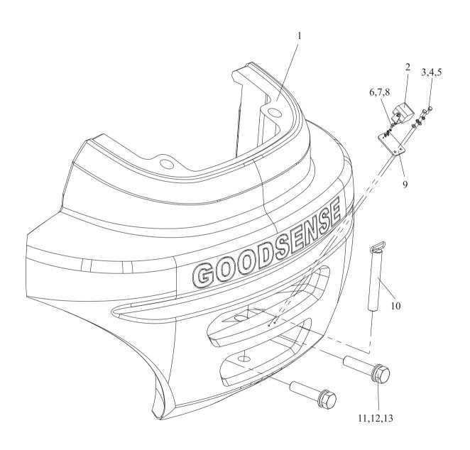
平衡重安装 Counterweight installation
